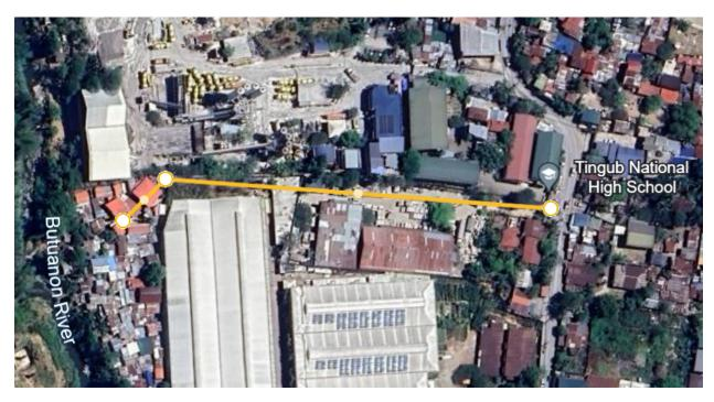
The proposed solution is to be implemented at the edge of the residential area in Purok I and over the narrow roads leading to Tingub National High School. The first station of the proposed cable transportation system is located at the red dot as seen in the image above and will then go to the top of the hilly area, where the second station is located. Then it will go downhill
